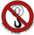
Do Not Lift Equipment with Hook – No Lift Point
