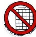
**Do not operate the compressor with the fan or coupling guard removed. Exposed fan and coupling may cause personal injury.**
