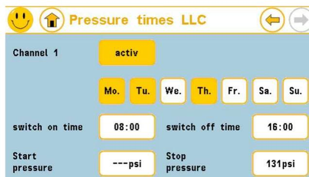
Figure 20: Page 1 of channel settings for times for basic load cycle priorities.
