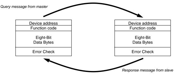
Shown below is a typical Modbus message structure. The values of the Modbus message are expressed as hexadecimal with certain values paired as shown. The Modbus message elements are defined in the following chart.
