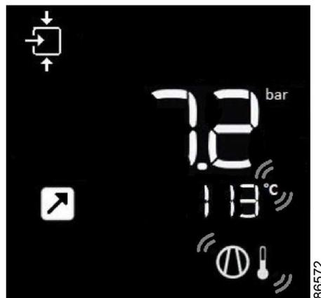
Figure 4: Main screen with temperature outlet warning
