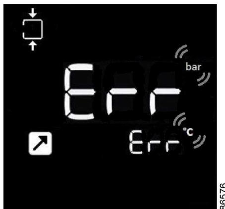
**Figure 8: Error on pressure and temperature sensor**
