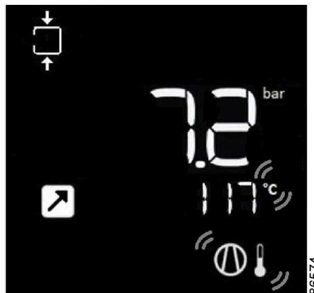
Figure 6: Main screen with temperature outlet shutdown
