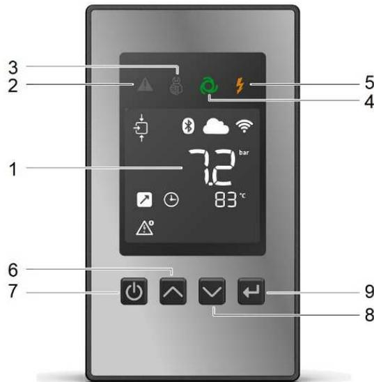
Service mode can be only enabled/disabled physically on the controller, this function will allow to notify the customer on the App that the service has been started on the machine and when it will be finished. It will also prevent remote start/stop when a service technician is working on a machine.
