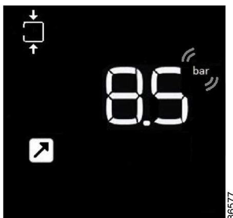
**Figure 9: High outlet pressure**
