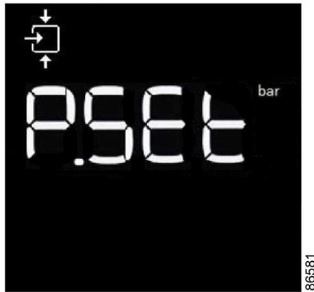
Figure 13: Pressure setting screen
