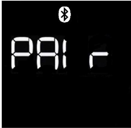
**Figure 19: Bluetooth pairing screen/ discovery mode**
