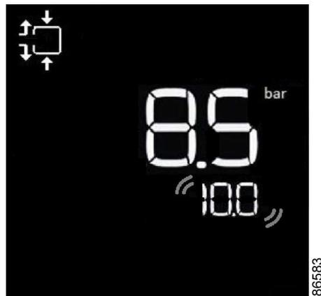
**Figure 15: Stopping/unloading pressure changing**
