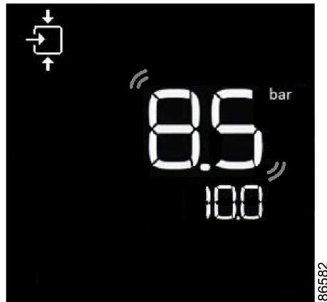
**Figure 14: Starting/loading pressure changing**
