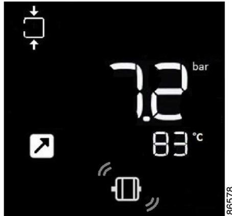
**Figure 10: Main screen with shutdown indication, motor overload**
