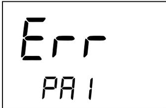
The message **-Err-** blinks for about 3 seconds to indicate the password code is wrong and shift back to the main visualization.
