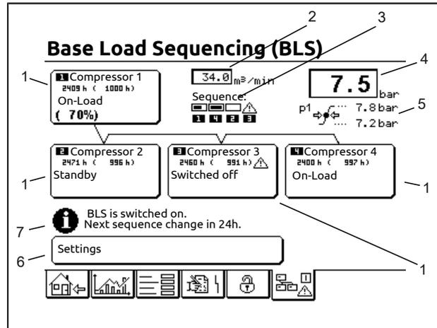
Fig. 10-4: Menu "Base Load Sequencing (BLS)" (typical display)
