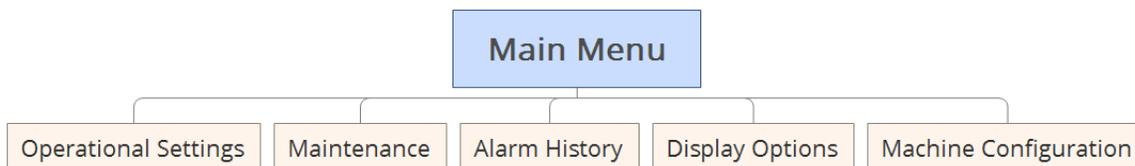
The default values for the adjustable parameters are determined by the compressor model configuration stored in the controller's memory. Most of these parameters can then be reconfigured if necessary by accessing the appropriate submenu within the *Main Menu*. Section 5.1 details the functions and parameter settings found within this top level menu.
