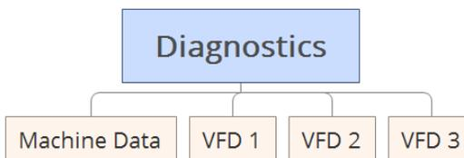
Selecting *Machine Data* will yield three pages. The first page shows compressor temperature readings, such as high temp fault, high temp alarm, discharge temp, inlet temp, oil temp, etc. The second page shows compressor pressure readings, such as high pressure fault, high pressure alarm, unload pressure, load pressure, etc. The third page shows plant delivery pressure, reservoir pressure, differential pressure, and separator pressure.
