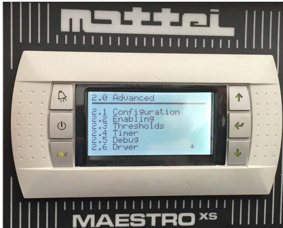
Step 13. Using down arrow scroll to screen 2.2.2 and press “enter < ↵ > key”. scroll to “Network” and place check mark on yes using “up” arrow key and “Enter” for “Network”. Then press “esc”
