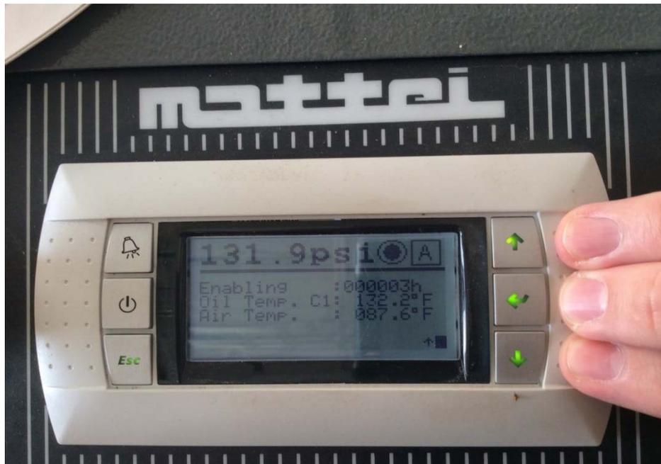
Step 3. Change **ONLY** the “Display address setting” number to “00” by pressing “enter < ↵ > key” and then the “up” arrow.
