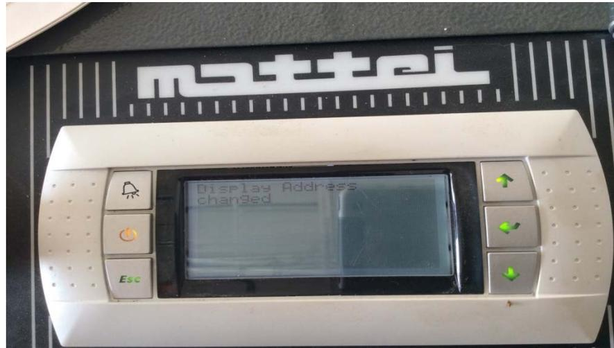
Step 5. **Turn power off.** After 30 seconds power compressor back on and after 2 seconds press the “bell”(reset) and “up arrow” keys simultaneously and hold until “Self Test” displays and wait
