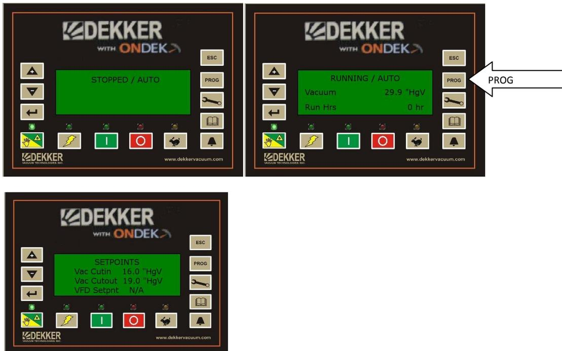
Press UP or DOWN button if necessary to select Vac CutIn then press ENTER
