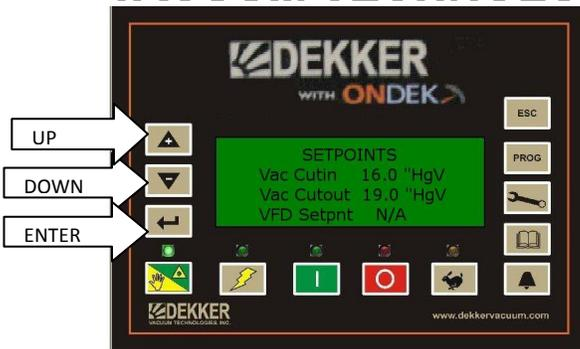
Once ENTER is pressed use UP or DOWN arrows to change value then press ENTER to save. Using UP/DOWN arrows repeat for Vac CutOut and save again by pressing ENTER
