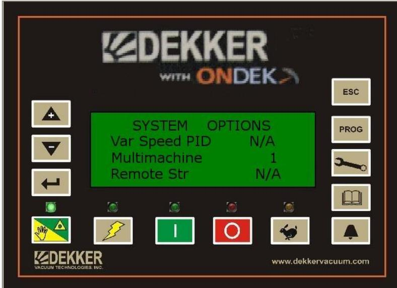
Go to second Controller Enter Password and follow same steps above only change multimachine to 2 and press ENTER.
