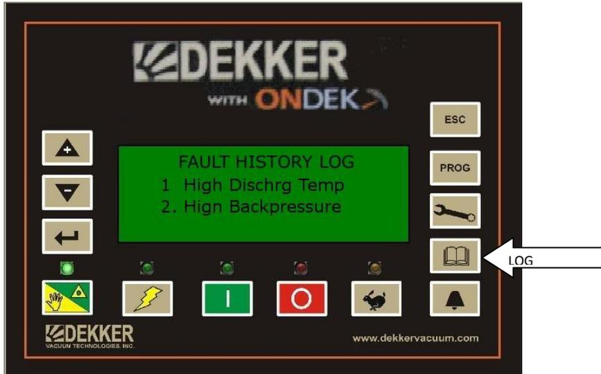
Each fault can be selected to view what values such as Vacuum, Back Pressure etc... were at the time of the fault and up to 10 minutes prior to the fault.
