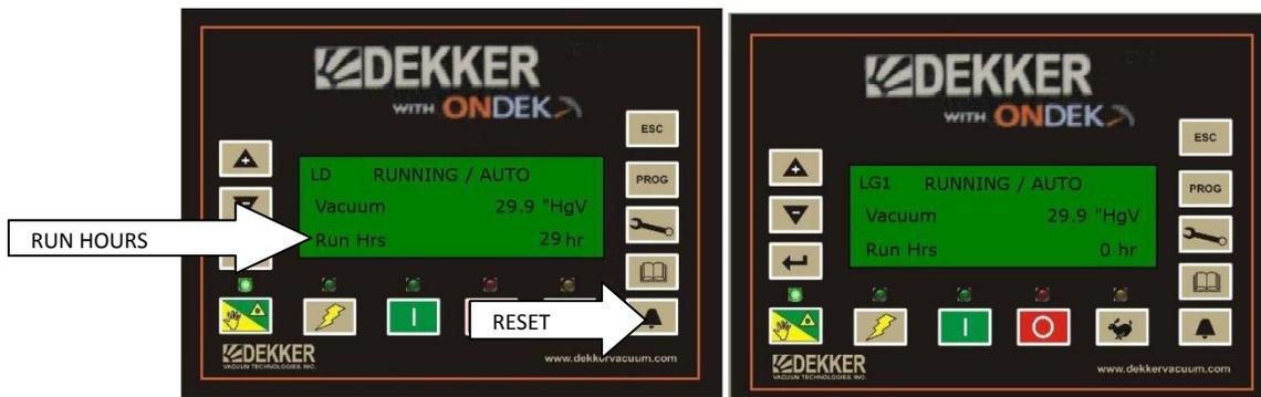
To rotate pumps manually, On the Lead pump, press and hold RESET button until you see the text “Manual Transfer” appear on the screen, then release the button. Wait a few seconds and you will see the upper text “LD” move to the opposite controller, the text “LG1” will move to where the “LD” was previously.
