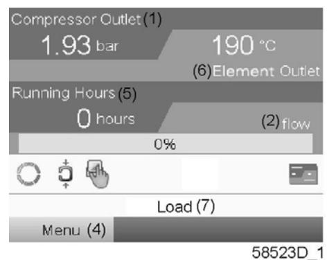
Typical Main screen (4 value lines), compressors with frequency converter
