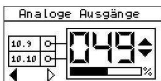
By means of the ▼ or ▲ key the analogue output can be set, whereas 0 - 100% corresponds to output type 0...10V, resp. 4...20mA .
