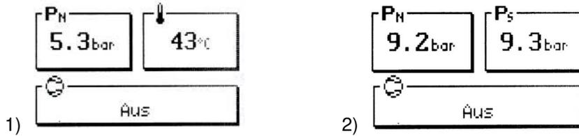
This is the main display in the control menu. Here the net pressure, the final compression temperature and the compressor status are displayed (1).
