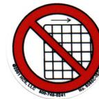
**Do not operate the blower with the fan or coupling guard removed. Exposed fan and coupling may cause personal injury.**
