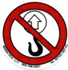
Do Not Lift Equipment with Hook – No Lift Point
