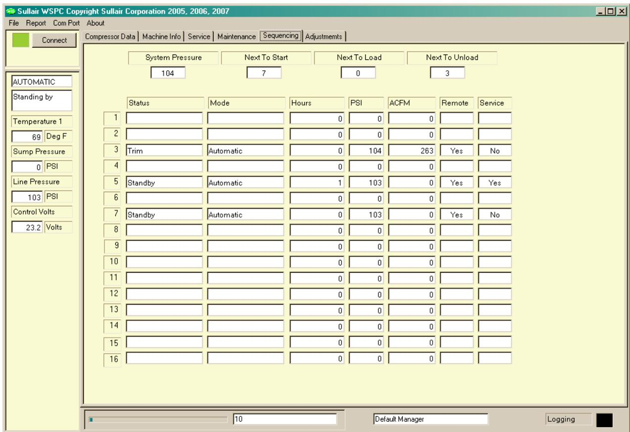
**Figure 3-2: WS Controller sequence system display**
