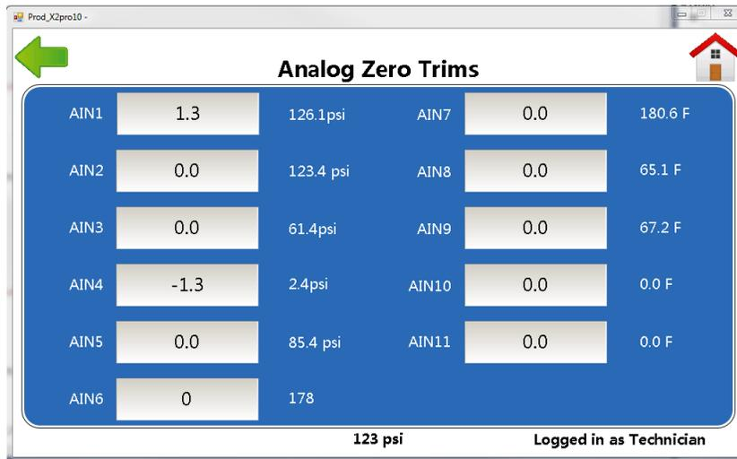
Figure 3-4: STS controller Analog Zero Trims
