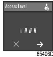
The user can enter the password by swiping up or down on the right vertical swipecover to select the first digit.
