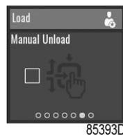
Manual unload can only be activated when the machine is in LOAD and Local control.
