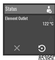
To reset the alarm, press the confirm button under the reset icon.
