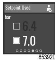
To switch to a different setpoint, swipe up or down on the left vertical swipebar or tap next to the corresponding square.
