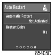
The controller has a built-in function to automatically restart the compressor when voltage is restored after voltage failure. This function is deactivated in compressors leaving the factory and can only be modified after entering a password, please consult your supplier to activate this function.
