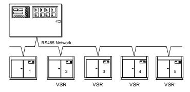
Integration with a CMC air system management controller is inherent to all R1 controllers.
