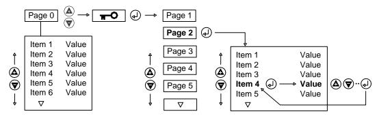
Press ESCAPE at any time in menu mode to step backwards one stage in the navigation process. Pressing ESCAPE when the page number is flashing will exit menu mode and return the display to normal operational mode; page 0.
