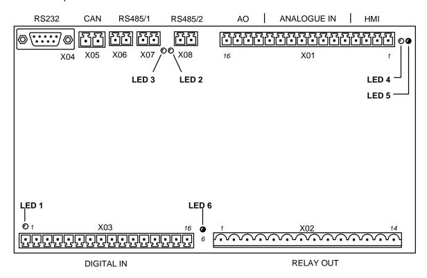
LED's 1-4 use different system timers and predefined blink rates to indicate different active functions:
