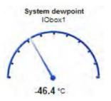
Analogue input name, location, value including unit of measurement displayed on a scaled 'qauge' indicator.
