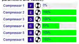
Below the Metacentre™ system controller 'status area, each compressor connected to the Metacentre™ system controller has a dedicated view area. The monitoring of compressor status, condition and event triggers can be monitored from here...
