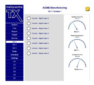
Three 'I/O' screens are provided; I/O 1, I/O 2 & I/O 3. The purpose of each screen is to provide individual I/O environments (e.g. 'Compressor house I/O monitoring' or 'Factory Line 1 I/O monitoring').
