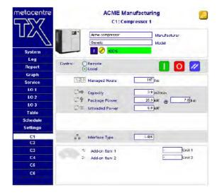
The number of visible 'C' compressor navigation buttons will correspond with the number of compressors configured as part of your Metacentre™ system installation.
