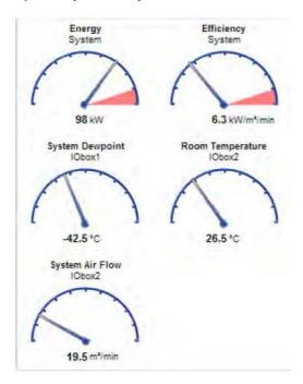
Up to 6 gauge displays can be viewed at the system home page. 'Energy System' and 'Efficiency System' are derived by calculation and/or from a physical flow meter if connected to the Metacentre™ system. Both gauges seek to provide an indication of total system efficiency.
