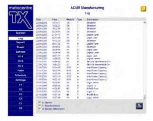
The Log screen retains a historical log of Alarm/Warning (A), Trip (T) and system (S) event conditions. Each event is logged chronologically, most recent first. You can filter event conditions by selecting the appropriate filter at the bottom of the log page.
