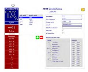
On the Accounts screen you can create new, modify existing and remove User accounts as well as set remote message filters.
