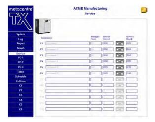
Service screen is Metacentre™ Cyber Console's scheduled service adviser. Use this to set up when service (routine maintenance) is due on each air compressor connected to the Metacentre™ system controller. Remote service Due messages can be generated (see User Accounts, configuration).
