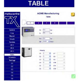
Depending on the Metacentre™ system controller in use, up to 6 tables are accessible.
