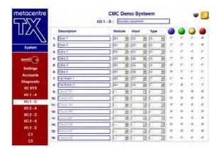
There are three individual I/O screens (I/O 1 to I/O 3). Each screen can be configured with up to 16 Digital indications.
