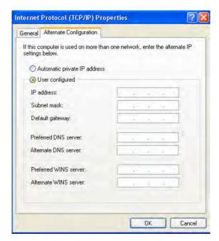
Select 'Alternative connection' and then select 'User configured'. Assign the computer an IP address of 192.168.1.3 and a sub mask of 255.255.255.0 – leave all other settings blank.
