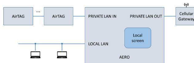
Figure 17 - LAN connections on the AERO
