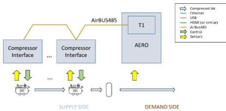
Figure 23 - AERO 'T1', AirBUS485, compressor interfaces
