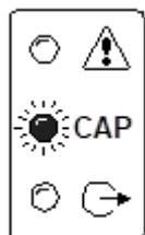
Figure 133 - Insufficient Capacity Alarm
