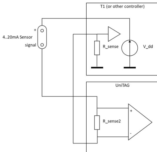
Figure 162 - Routing of the pressure sensor currents
