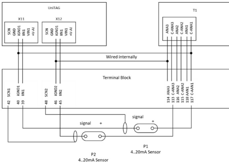
Figure 163 - Wiring of the P1 and P2 sensors
