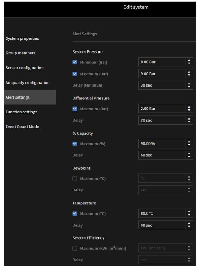
Figure 109 - Alert Settings - configuration in AirCloud
