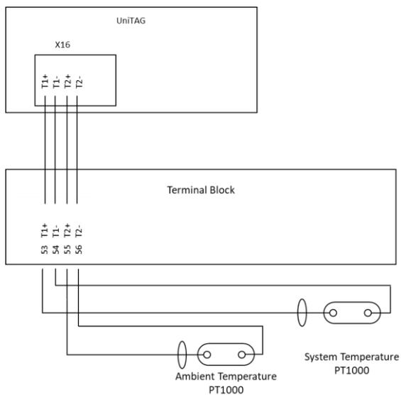
Figure 165 - Connection of Temperature Sensors
