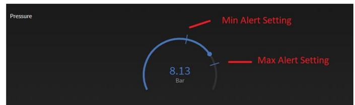
Figure 84 - Alert setting: both Minimum and Maximum Alert levels are set
