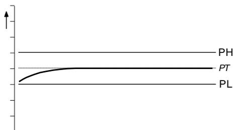
Figure 113 - Variable Speed compressor targets PT
