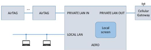
Figure 29 -- LAN connections on AERO – standard use
