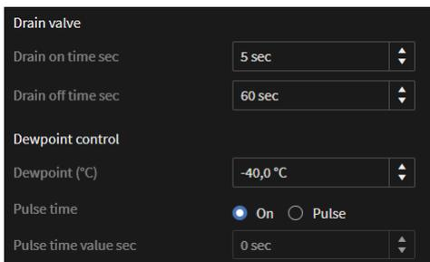
Figure 156 - Configuration of Relay 2 and 3 on UniTAG
