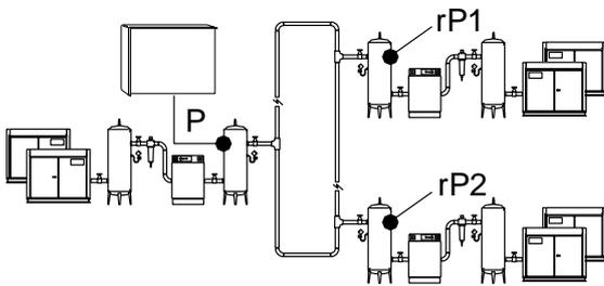
**!** Remote pressure references are transmitted on the RS485 network at maximum intervals of ten seconds. If RS485 communications is disrupted the management unit will automatically default to using the primary pressure for control.
