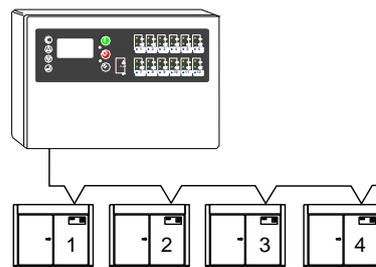
Figure 146 - Compressor identification for the T1
