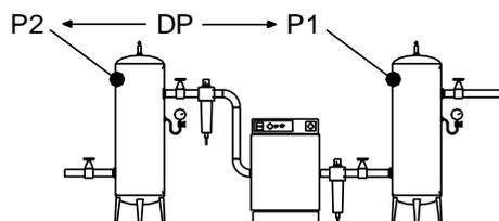
Figure 130 - 2nd Pressure Sensor - Differential mode
