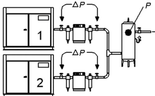
Figure 20 - Control Pressure Sensor Location, Demand side
