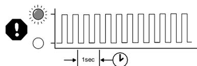
The Fault LED will 'fast flash' to indicate a Trip (Shutdown) condition.
