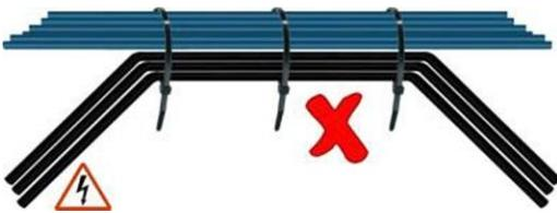
Figure 12 - How not to place cables
