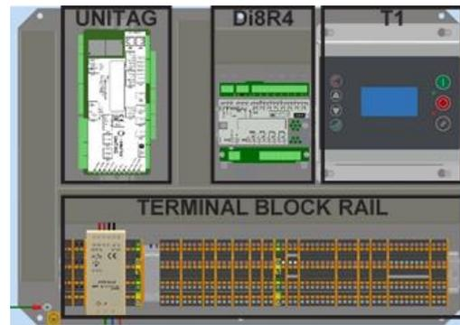
Figure 8 - Components located on the back-plate
