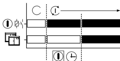
Figure 127 - Auxiliary equipment pre-started prior to compressor utilization
