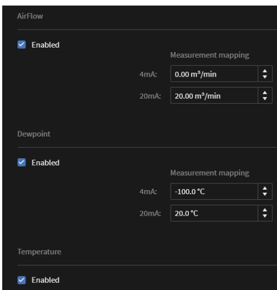
Figure 103 - AirCloud based Sensor configuration for UniTAG in AERO – part 2
