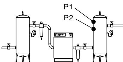
Figure 129 - 2nd Pressure Sensor - Backup Sensor mode
