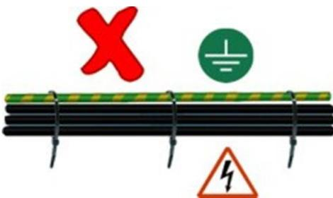
Figure 13 - How not to place cables part 2
