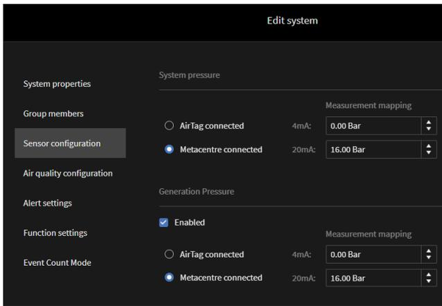
Figure 102 - AirCloud based Sensor configuration for UniTAG in AERO – part 1
