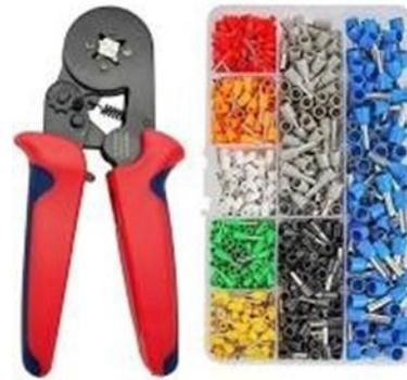
Figure 15 - Cable tooling
