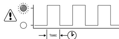
The Fault LED will 'slow flash' to indicate an Alarm (Warning) condition. An Alarm (Warning) indicates that the AERO is continuing with normal operation but user attention is required.
