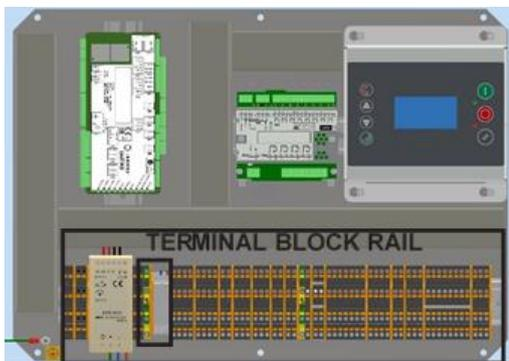
Figure 16 - power supply connection location
