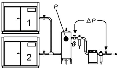
Figure 19 - Control Pressure Sensor Location, Supply side
