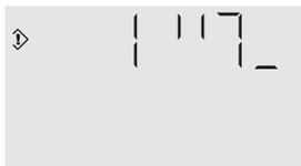
After an output phase the compressor switches to an idling phase before decreasing the system pressure and finally switching into stand-by. For compressors with special ventilation an additional after-running time is necessary to avoid the formation of condensate in the compressor. The after-running time can be adjusted as follows:
