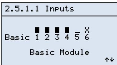
If we enter the submenu [Advanced\Debug\Inputs] the page to the left will be displayed. It shows the state of the digital inputs of the base module of MAESTRO xs.
