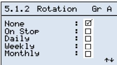
If we select the “Sequence” mode we can select programmed rotation of the first compressor to be started up when the group A network is enabled. This rotation may be:
