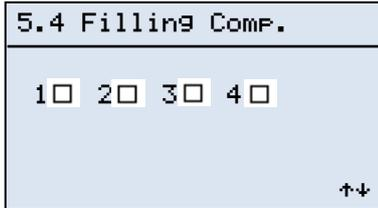
We can select a compressor for filling the line. The display shows the n compressors available in the network, but we can only select one compressor for filling the line.
