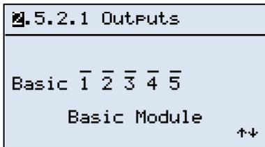
once you are in the output enabling menu press the <↓> key to test the outputs on the base module, or the <↓> key to go to the expansions page.
