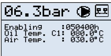
If the compressor is enabled as "Slave" the operating icon will be as shown on the left.
