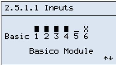
This first page checks the state of the digital inputs on the base module of MAESTRO xs.
