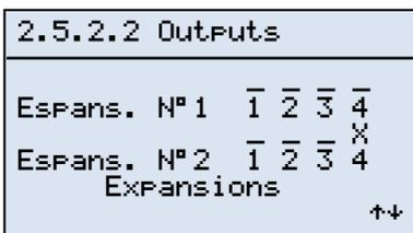
On the second page, which can be seen only if one or both of the expansion modules is enabled, we can activate the digital outputs of each expansion.
