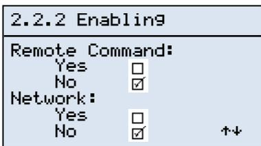
To enable the use of remote enabling/disabling, we must select “Yes” in the [Remote command] function of the [2.2.2 Enabling] menu. Now carry out the primary enabling, from the keyboard, by pressing the <On/Off> key.
