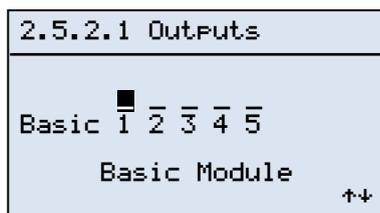
Pressing the <↓> key takes the cursor to output N°1, and then pressing the <↑> key activates the output.
