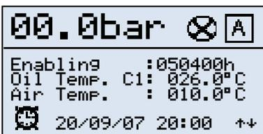
Ronan weekly programming is active a clock icon is displayed on the screen. To exclude programming we can proceed in two ways. The first is to go to the clock menu and deactivate the selected mode. The second involves pressing the <↵> key for five seconds: the clock icon will start to flash, telling the user that programming has been excluded.
