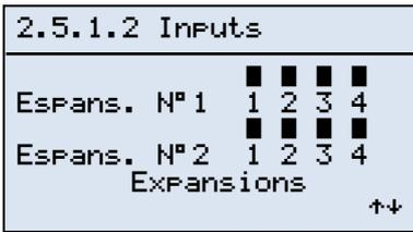
on the second page, which is visible only if one or both expansion modules are enabled, we can monitor the four digital inputs of each expansion.
