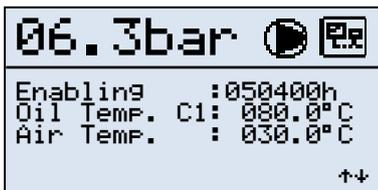
If the compressor is enabled as "Master" the operating icon will be as shown on the left.
