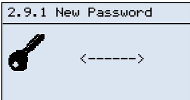
The new password must be created with a combination of the Up and Down keys.
