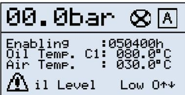
This is an example of a fault report: in addition to a description of the type of fault the user is told that the compressor is in "BLOCK".
