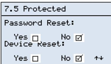
The display on the left makes it possible to “reset” the access password for the “service” menu, restoring the password predefined by Mattei.
