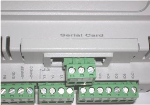
Once the board is installed connections must be made to the extractable terminals. The final configuration is shown on the left.
