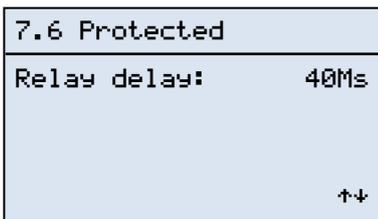
the display on the left makes it possible to modify the delay times of the commutation of the starring triangle contactors.
