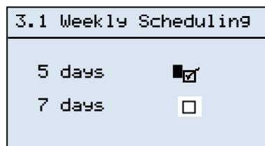
Once you have made the selection press the <↓> or <↑> key to enable the function. A check mark will be displayed showing that the required function has been selected (e.g. 5 day mode).
