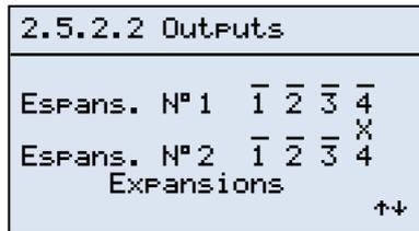
When we enable the first expansion of the system the page on the left will be displayed; it shows the logical state of:
