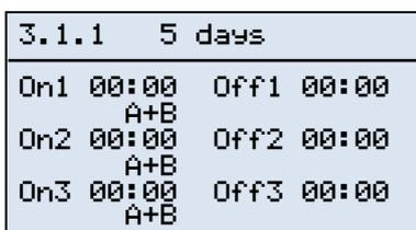
If we enable the network mode on the compressor configured as Master, the timer configuration page on the left will appear.
