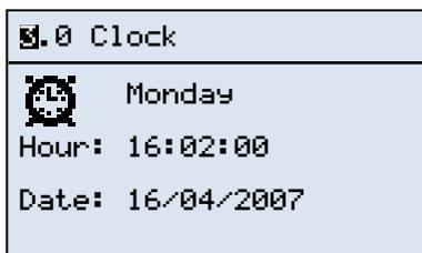
to enable weekly programming we must go to the [Clock] menu. We will see the flashing cursor on the first character at the top left of the screen, and from here we will use the <↓> key to access the page where programming is enabled and selected.
