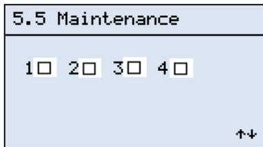
The final page of the menu allows us to exclude one or more compressors from the network to enable maintenance.
