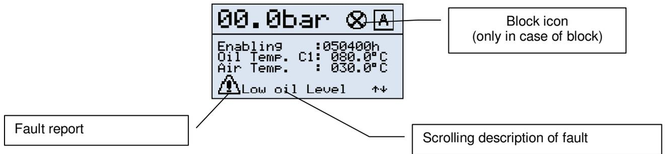
On the first page of the [Monitor] menu, an icon is displayed at the bottom left showing the presence of a fault on the compressor; alongside it is the description of the fault. This description scrolls to allow a complete report to be given.
