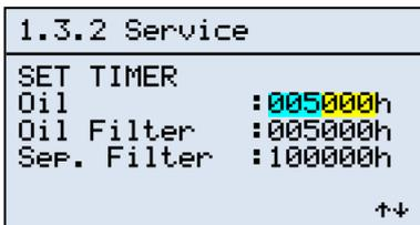
Before describing the hour counters we must explain that every hour counter is divided into two parts, as shown in the figure on the left, which permits quicker and easier modification when configuring the counter.
