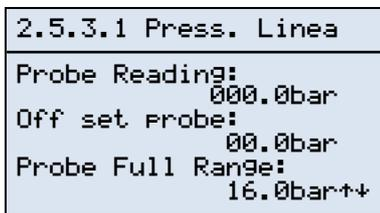
By entering the [Advanced\Debug\Pressure Probes] submenu we can configure the pressure probes on the machine. The display is divided into two pages (one per probe) structured as shown on the left.
