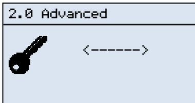
As already mentioned, a password must be entered to access this menu. The password is a combination of six numbers, entered by pressing the arrow keys.
