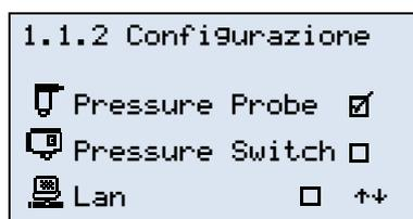
MAESTRO xs can control the compressor using a pressure probe or a mechanical manostat.
