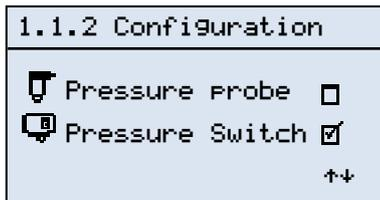
For this kind of operation, access the “1.1.2 Configuration” menu page, move the “Pressure probe” selection to “manostat” and then use the On/Off key to enable the machine.
