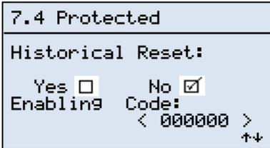
The display on the left permits the Log of the controller to be “reset”, but not including the number of start-ups, which can be reset to zero only by completely resetting the unit.
