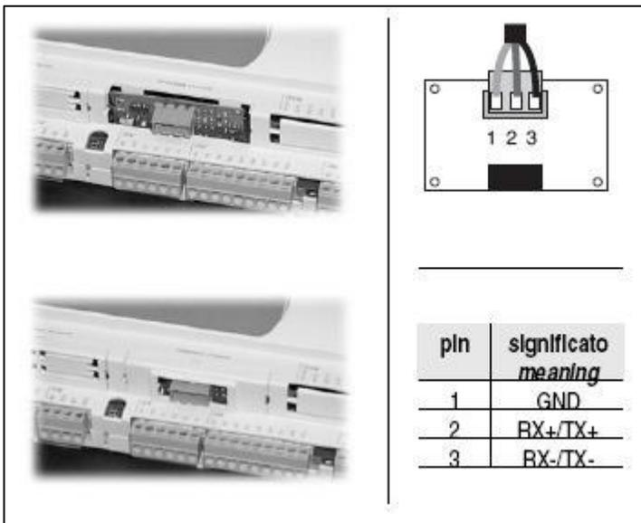
On the left is the correspondence of the electrical connections of the serial board.
