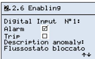
When the fault description is complete the cursor will return to its original position; we can then go to the description of the next digital input or return to the preceding menu.
