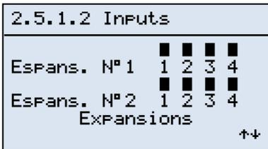
If the second expansion of the system is enabled, the screen on the left is displayed. It indicates the logical state of:
