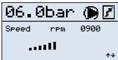
When the Optima mode is enabled the page on the left showing the rotation speed of the compressor is displayed.
