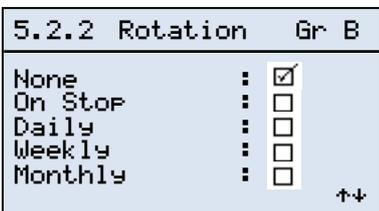
For group B too, if we select the “Sequence” mode we can select programmed rotation of the first compressor to be started up when the group B network is enabled.
