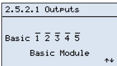
When we enter the [Advanced\Debug\Outputs] submenu overpaid shown on the left is displayed. It allows us to "force" the individual digital outputs of the base module of MAESTRO xs.
