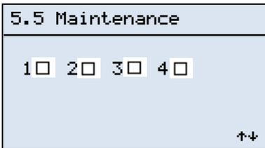
On the final page we can inform the “Master” that compressor n has been removed for maintenance.
