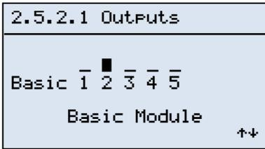
it is possible to activate one specific output by pressing the <↓> key until you reach the desired output and then pressing the <↑> key to activate it.
