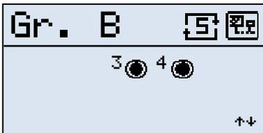
In this display, which will appear only if we have divided the compressors into two groups, we can see the working mode of “Group B”.
