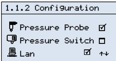
If we enable the compressor to operate in “Network” mode the 1.1.1 configuration page will no longer be accessible, while page 1.1.2 will display a third icon as shown on the left.
