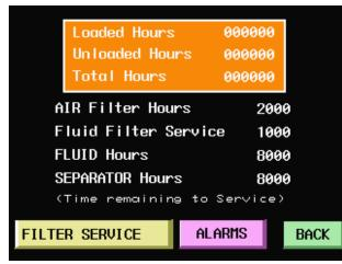
This screen displays the loaded, unloaded and total hours on the compressor as well as the remaining hours until service is required based on the service hours settings.
