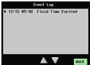
The Event Log screen displays all of the service and shutdown events that have occurred on the compressor. Up to 200 events (with date and time) can be recorded. Press the up and down arrows to scroll through the events.
