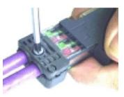
Loosen the screw of the strain relief on the connector, turn back the strain relief clamp and lift the contact cover.
