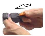
Mark the position using the index finger of the left hand and insert the cable into the tool (to the measured distance) and clamp the end of the cable in the stripping tool as shown.
