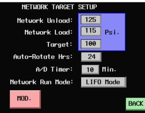
Set the Network Unload pressure, Network Load pressure, Target Pressure, Auto-Rotation Hours, Auto-Dual Timer, and Network Run Mode (press the gray box next to Network Run Mode to toggle from LIFO Mode to Auto-Rotate Mode). Reference page 24 for a detailed explanation of these settings. All of the network settings are transmitted to all active compressors on the network.
