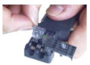
Once the cables are properly installed in the connectors, plug the connectors into port 1 of the PLC.
