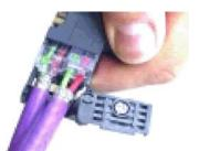
labeled A2, B2) and press the contact cover down firmly.
