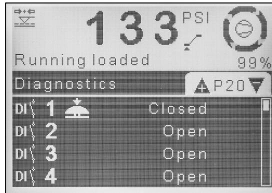
**Note:** Must not energize or de-energize relays in the Diagnostics. Serious damage can occurred to the compressor.
