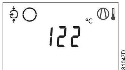
*The screen shows that the temperature at the element outlet is 122 °C*
