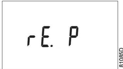
The function of this screen is to activate the remote load/unload relay. To be able to activate this remote Load/Unload functionality, a physical digital input with function Load/Unload is required.
