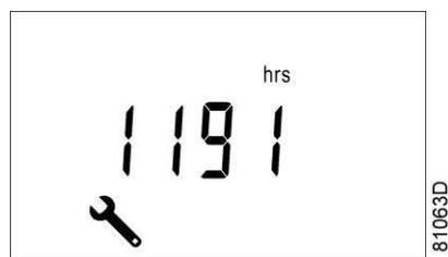
This screen shows the unit used <hrs> (or <x1000 hrs>) and the value <1191>. In the example shown, the compressor has run 1191 hours since the previous service.
