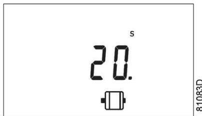
This screen shows the minimum stop time (20) and the unit <s> seconds.
