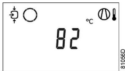
The screen shows that the outlet temperature is 82 °C.
