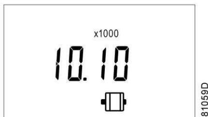
This screen shows the number of motor starts (x 1 or - if <x1000> lights up - x 1000). In the above example, the number of motor starts is 10100.
