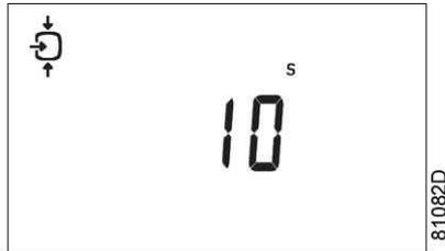
This screen shows the load delay time (10) and the unit <s> seconds.
