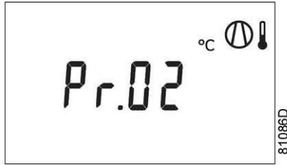
*Protection setting element outlet temperature*
