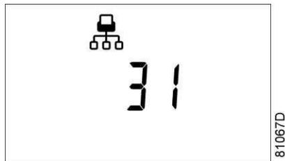
It is also possible to change the channels. The controller has 4 channels. When changing the channels, the controller can act as a Mk IV controller (a previous version of the controller). To set the channels, go to the screen where the node ID is visible.
