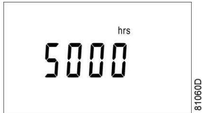
The screen shows the unit used (hrs) and the value (5000): the regulator module has been in service during 5000 hours.
