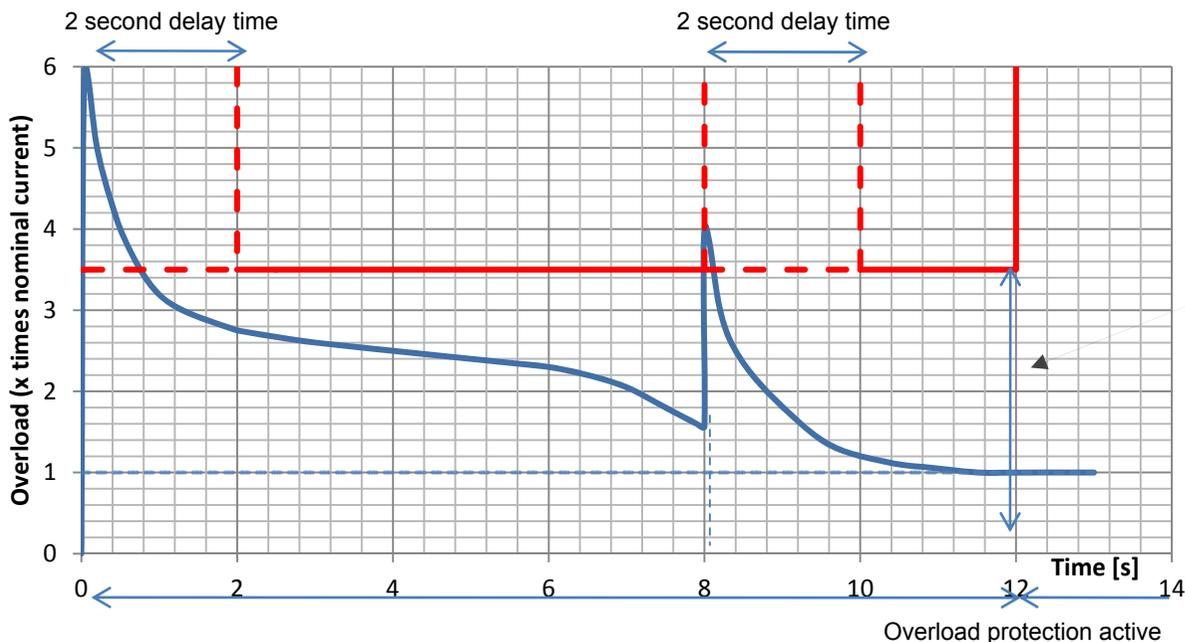
Main motor rotor lock protection level (Parameter P14.05)
