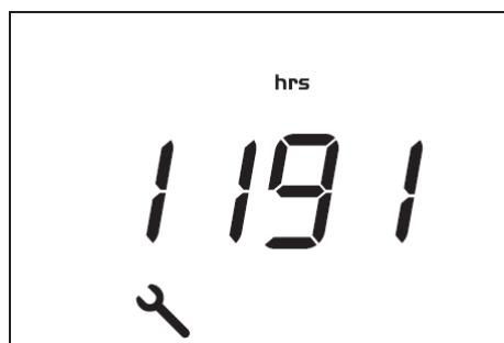
This screen shows the unit used <hrs> (or <x1000 hrs>) and the value <1191>. In the example shown, the compressor has run 1191 hours since the previous service.
