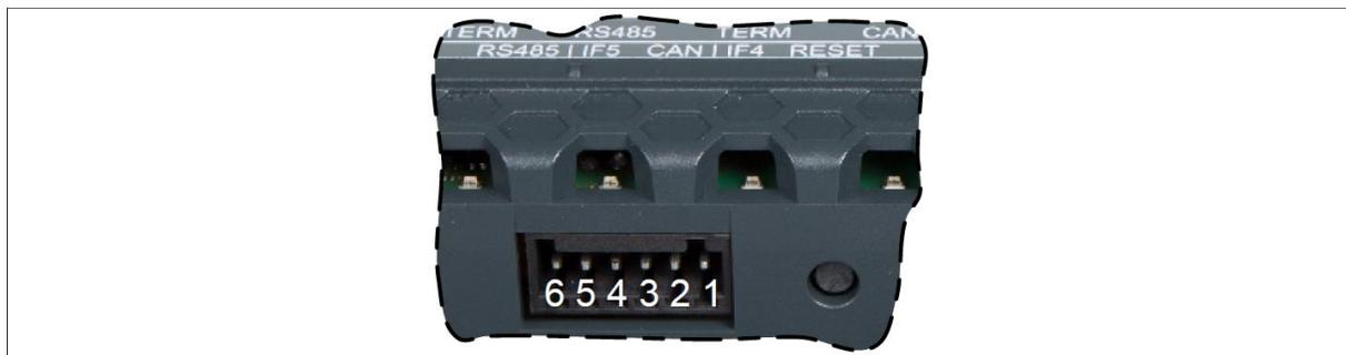
Figure 9: CAN bus and RS485
