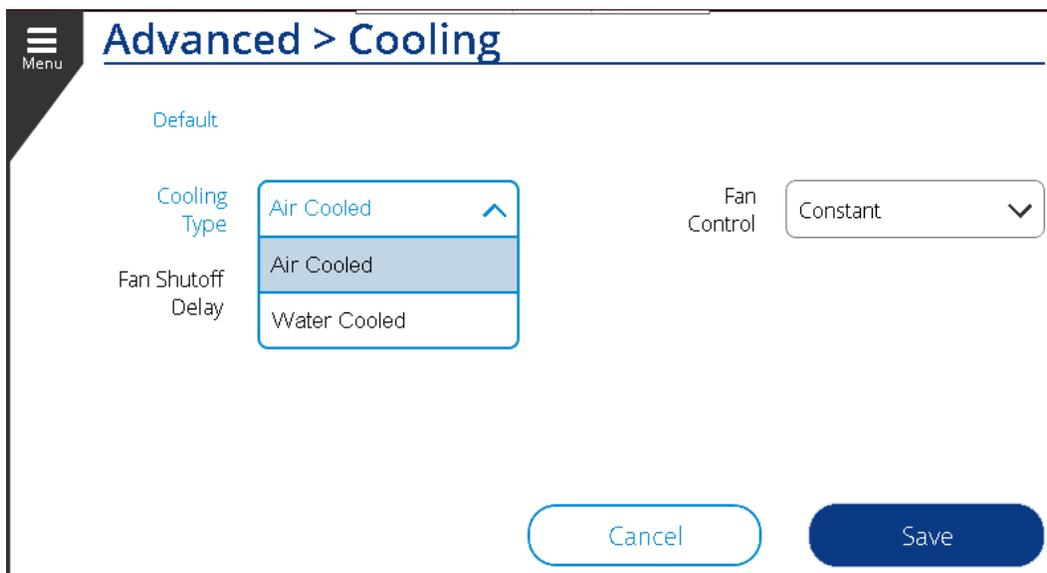
The screenshot shows the 'Advanced > Cooling' settings screen with the 'Cooling Type' dropdown menu open. The menu lists 'Air Cooled' (highlighted) and 'Water Cooled'. The 'Fan Control' dropdown menu is set to 'Constant'. The 'Fan Shutoff Delay' is not visible in this view. At the bottom, there are two buttons: 'Cancel' (light blue) and 'Save' (dark blue).
