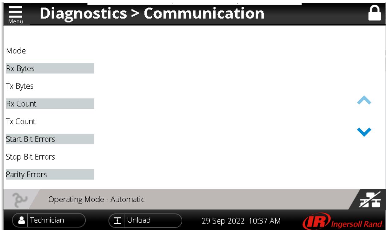
Figure 6.1-H: Communication Diagnostic Screens
