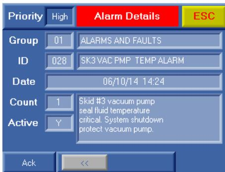
The Alarm Details screen shows all information about the chosen alarm. The Group, Group Name, ID, Alarm Name, Timestamp, Count, Active State and Alarm Description are shown. There is also an Acknowledge button at the bottom of the screen.
