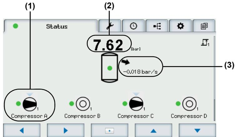
Fig. 4.4: Sub-view Master for multiple compressor system operation
