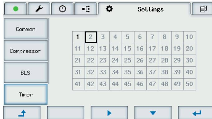
Fig. 4.12: Category "Timer" with 50 switch clock channels
