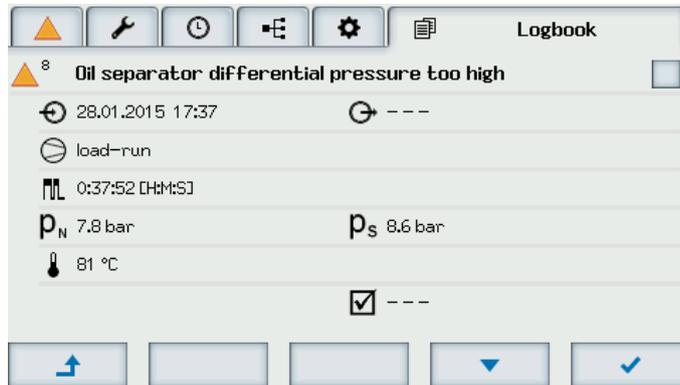
Fig. 4.15: Detailed view of a warning/service message
