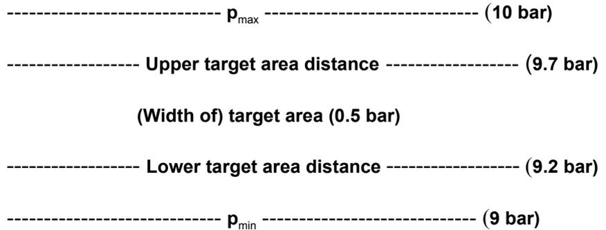
Fig. 4.11: Coherency pressure range – target area distance – target area width
