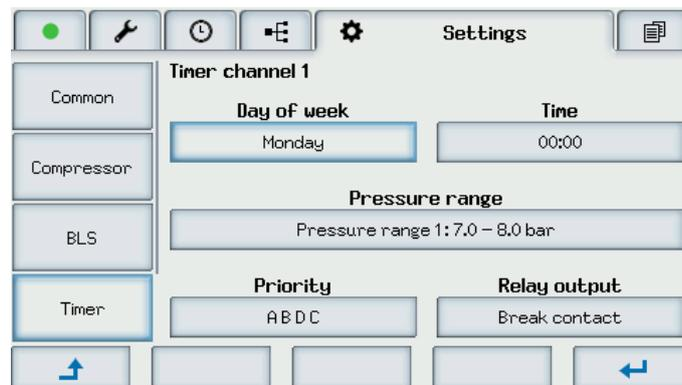
Fig. 4.13: Detailed view timer channel1
