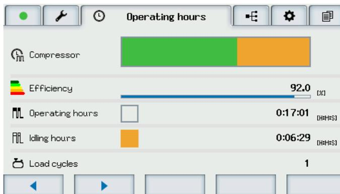
Fig. 4.7: Main display "Operating hours"
