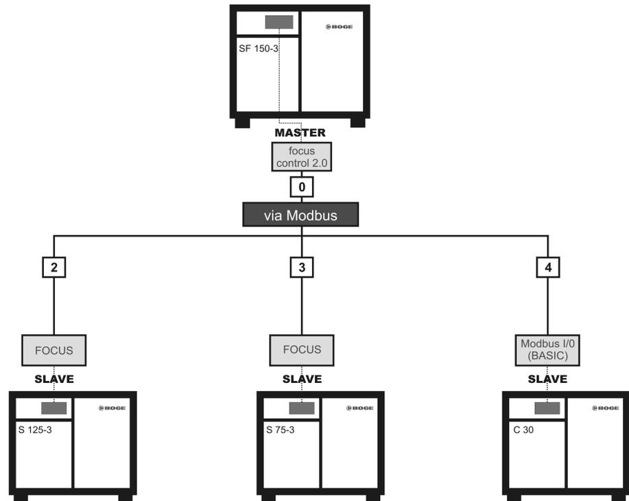
Fig. 3.1: **focus** control 2.0 as master control in a multiple compressor system – example
