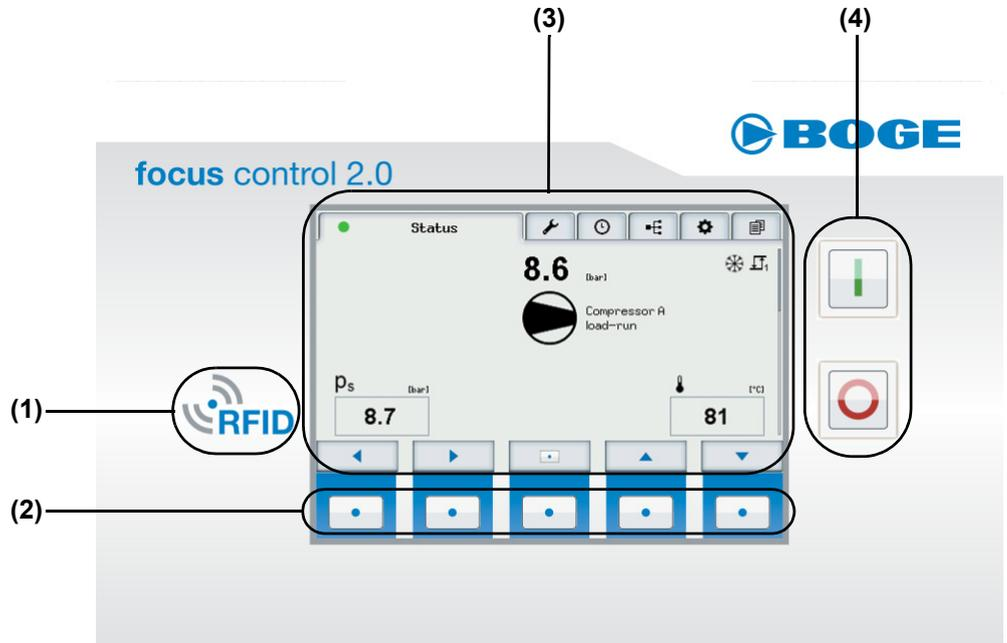
Fig. 3.2: **focus control 2.0** – Operating unit
