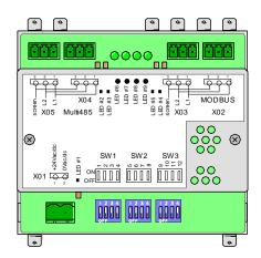
The Gateway Module (shown above), is supplied including 24vDC power supply; both for mounting within the host air compressors starter assembly.
