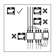
Avoid mounting the Gateway near high voltage cables, high voltage devices or equipment or motor starter contactors.
