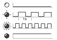
At power on initialisation, or when power has been removed, all operational indicators will fast flash for several seconds.
