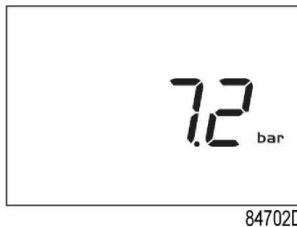
Main screen with pressure (stopped compressor)
