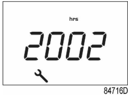
Example of running hours screen
