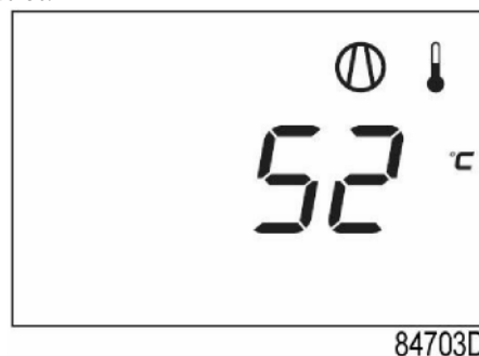
Main screen with temperature (stopped compressor)
