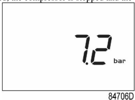
Main screen with pressure (stopped compressor)
