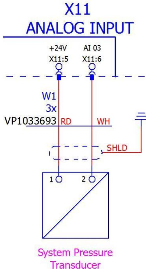
**Figure 4: System Pressure Transducer Wiring on IO Module using cable VP1033693**
