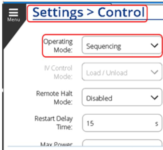
**Figure 37: Operating Mode Setting in Control Settings Menu**
