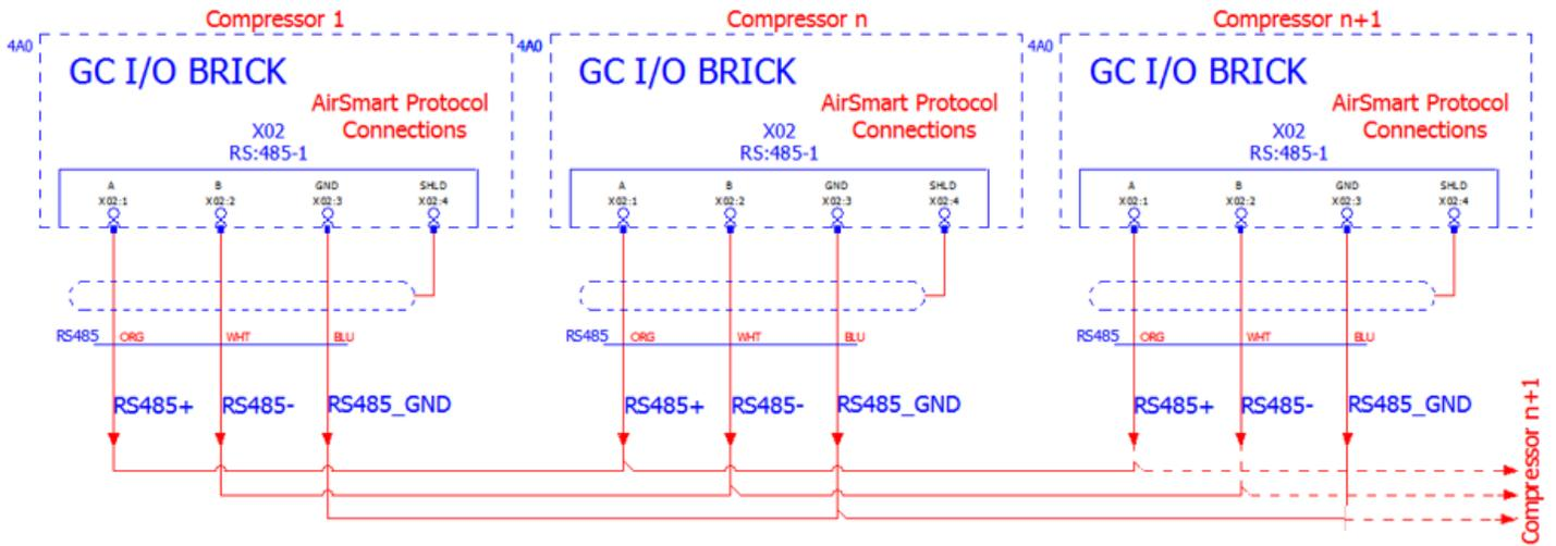
**Figure 5: AirSmart RS485 Communication Wiring Schematic**
