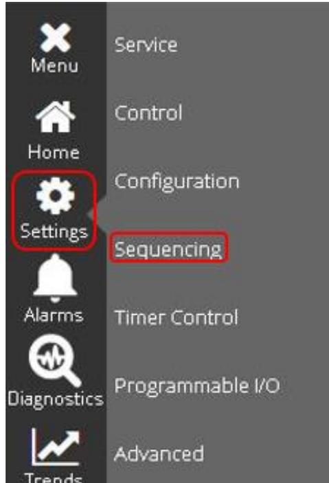
Figure 13: Menu navigation to sequencing screen
