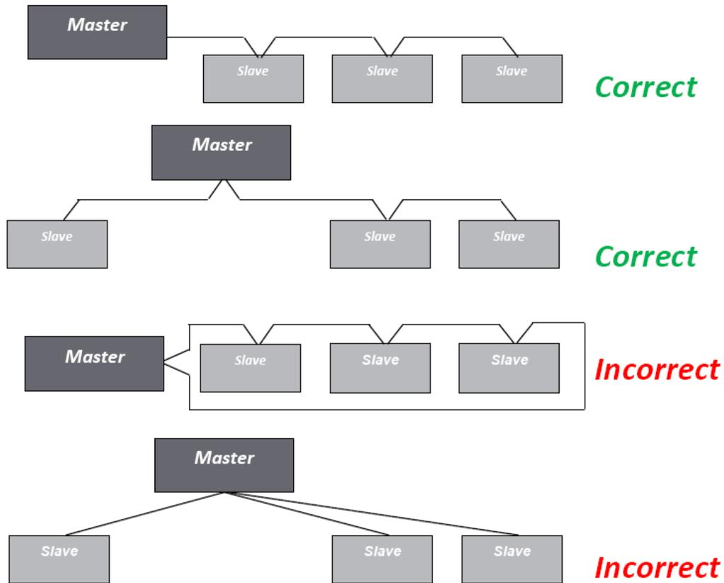
**Figure 3: Example RS485 configurations of the Master/Slave controls for communications**
