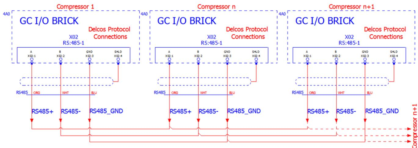
**Figure 18: Delcos RS485 Communication Wiring Schematic**
