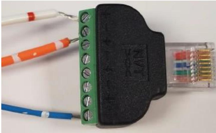
**Figure 7: Blue is RS485 GND, Orange is RS485+, White is RS485-**
