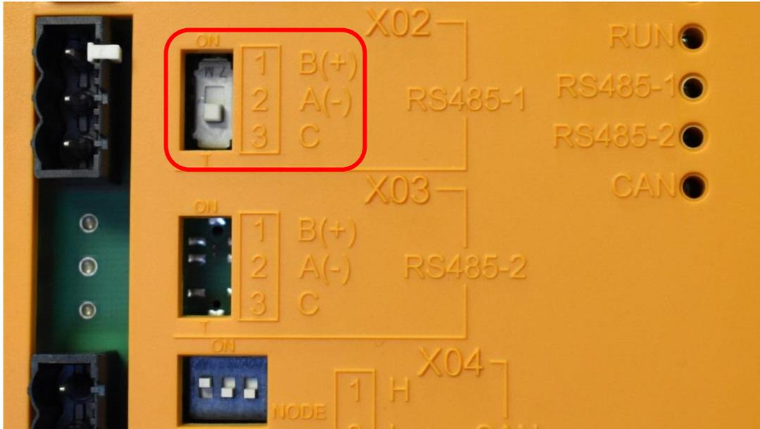
**Figure 19: IO Module DIP Switch Settings at RS485-1 Port**
