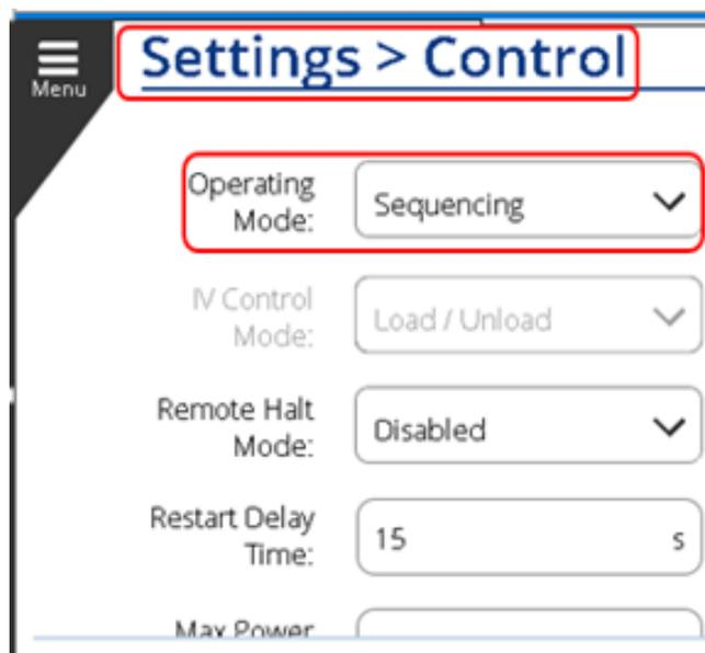
Figure 12: Operating Mode Setting in Control Settings Menu
