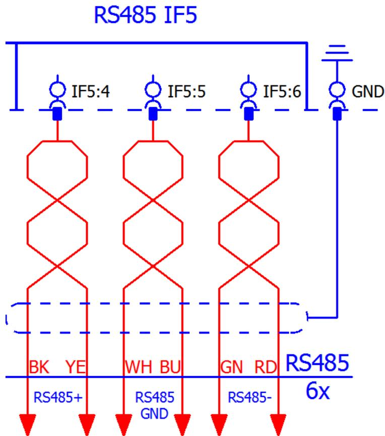
**Figure 32: Legacy ES+ RS485 Communication Wiring to Governor Display**
