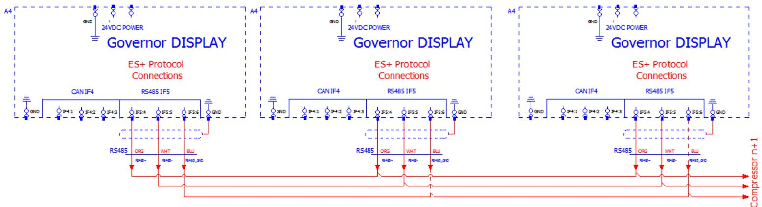
**Figure 31: ES+ RS485 Communication Wiring Schematic**
