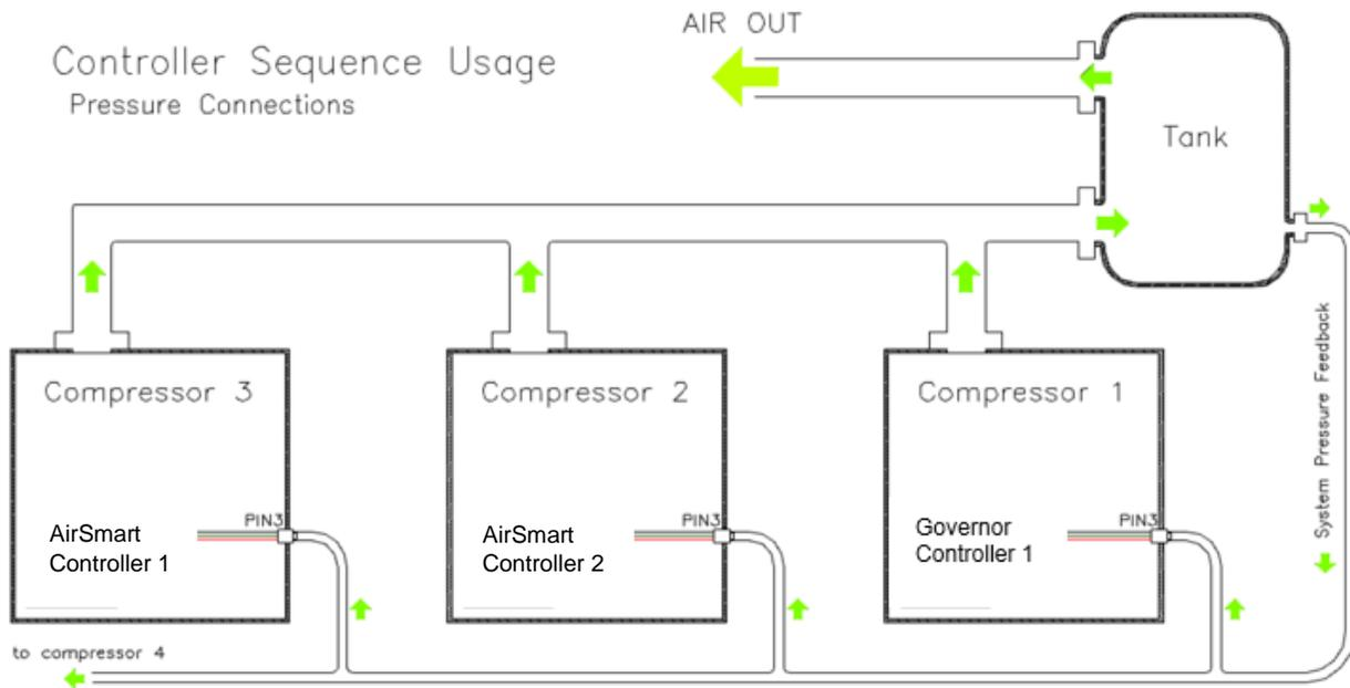
**Figure 1: Sequencing Pressure Connections**
