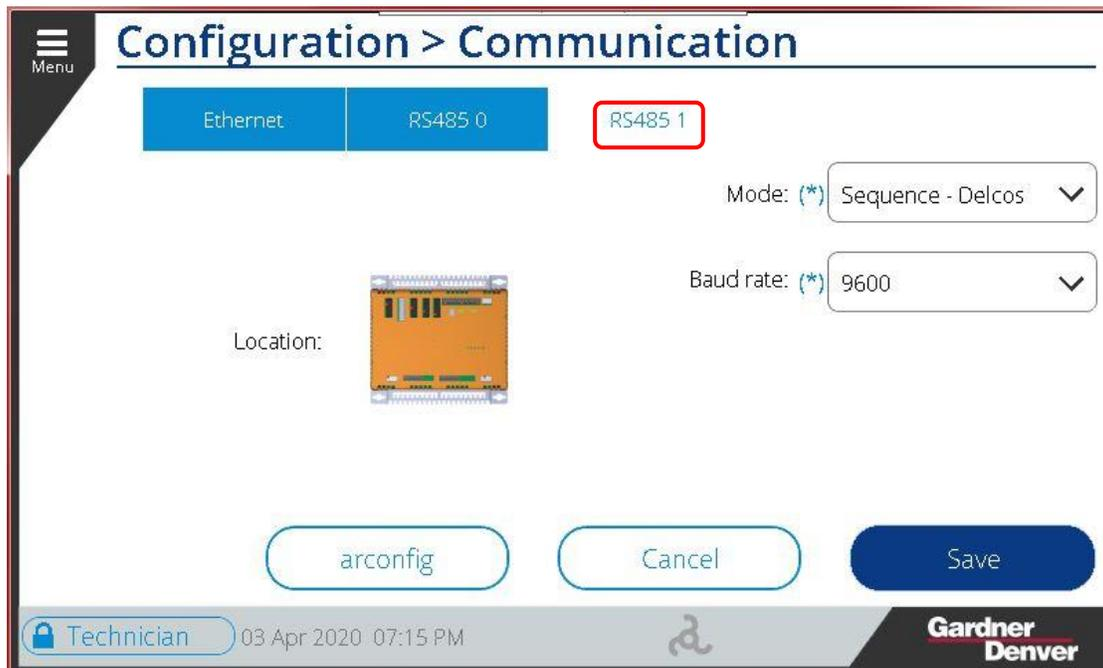
**Figure 21: Delco's Communication Configuration Screen**
