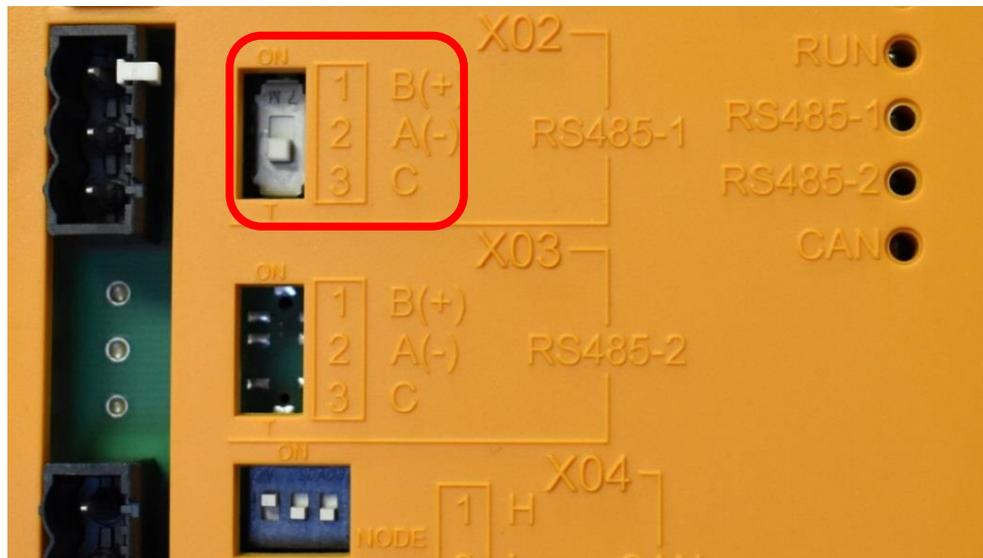
**Figure 6: IO Module DIP Switch Settings at RS485-1 Port**
