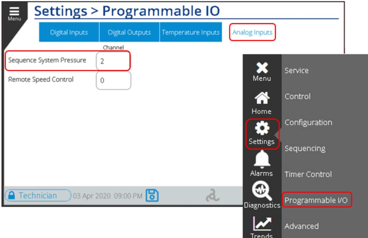
**Figure 15: Programmable IO Settings Screen**
