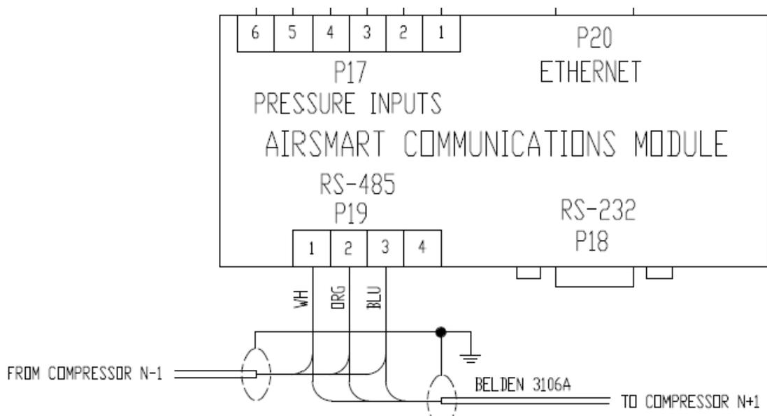
**Figure 8: Blue is RS485 GND, Orange is RS485+, White is RS485-**
