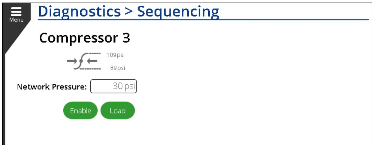
**Figure 28: Delcos Sequencing Diagnostics Page for a Slave**
