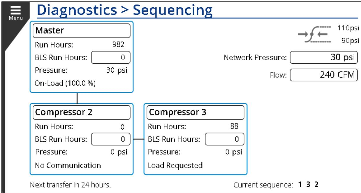
**Figure 27: Delcos Sequencing Diagnostics Page for a Master**
