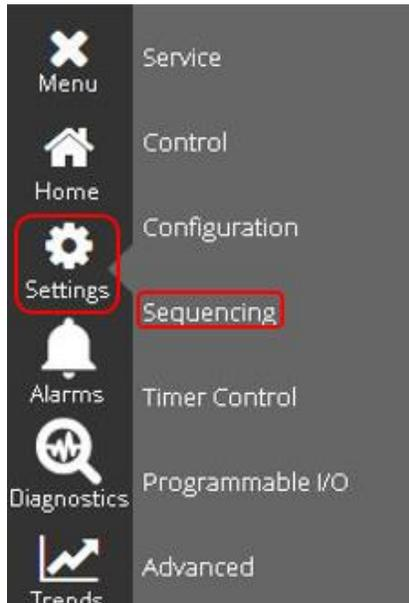
**Figure 38: Menu Navigation to Sequencing Screen**
