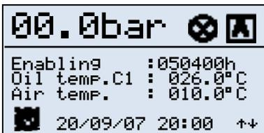
When weekly programming is enabled, a clock symbol is displayed on the monitor. To disable programming, proceed in one of the following ways. The first is to enter the clock menu and disable the selected mode. The second involves pressing < ↵ > for five seconds. The clock icon starts flashing to inform the user that programming has been disabled.
