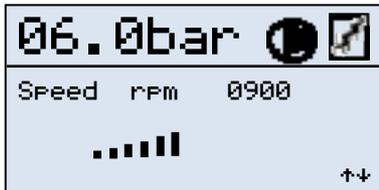
In the Optima mode, the page shown to the side, indicating at what speed the compressor is running, is displayed.
