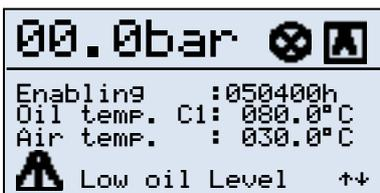
An example of a fault message is shown to the side where, together with an indication of the typology, the user is also informed that the compressor is "BLOCKED".
