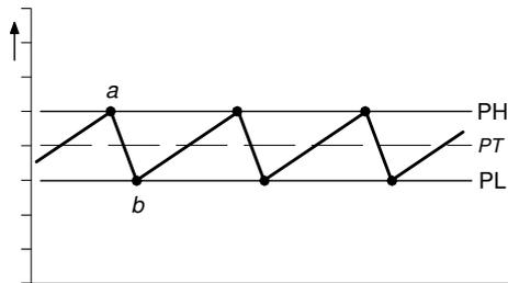
When system pressure increases to the High Pressure set point (a) a compressor is unloaded. Pressure is allowed to decrease to the Low Pressure set point (b) before a compressor is loaded again to add capacity output and increase pressure. This process will continue under a steady demand for air in a continuous stable cycle.
