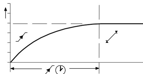
At system start (manual start or automated start from standby) the SX will only load compressors that have been pre-determined for prefill operation, for a pre-set period of time. The prefill time (PT) can be adjusted to suit system characteristics. The aim is to increase pressure to normal operational levels, using only the pre-determined compressors, prior to the prefill time expiring.
