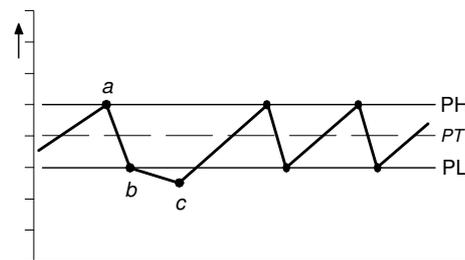
The same method is implemented in reverse (above the High Pressure set point) when an abrupt, or significant, decrease for air demand is experienced.
