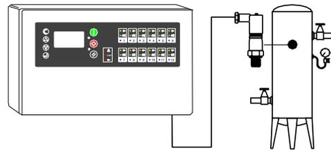
As default the EnergAir Metacentre SX is set-up for operation with a 16bar (232psi) pressure sensor but can accept input from any 4-20mA type pressure sensor with a range from 1.0bar (14.5psi) up to 600bar (8700psi).
