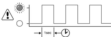
The Fault LED will 'slow flash' to indicate an Alarm (Warning) condition. An Alarm (Warning) indicates that the SX is continuing with normal operation but user attention is required. All Alarm (Warning) conditions are registered in the SX Error Log. All Alarm (Warning) conditions must be manually reset.
