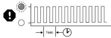
The Fault LED will 'fast flash' to indicate a Trip (Shutdown) condition. A Trip (Shutdown) condition will stop normal operation of the SX. Pressure regulation control will automatically revert to the individual compressors that will continue to operate using the pressure settings for their own control systems. All Trip (Shutdown) conditions are registered in the SX Error Log. All Trip (Shutdown) conditions must be manually reset.
