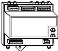
The direct connect interface module (i-PCB) is installed within the compressor control area and connected to the SX using a six-wire cable.
