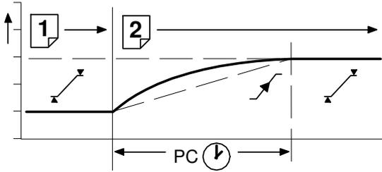
The time the system will take to complete the transition from one pressure target to another is determined by the 'Pressure Change' time (PC). This value can be adjusted to accommodate installation characteristics to achieve the transition at optimal energy efficiency.
