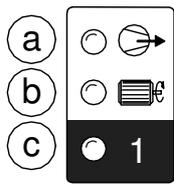
Each compressor in the system has a set of dedicated status indicators. The indicators will continuously show the status of each compressor at all times.
