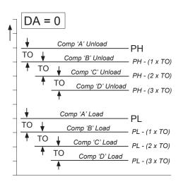
It is permissible for the 'Unload' and 'Load' levels to overlap if the 'PH' and 'PL' levels are set close together.
