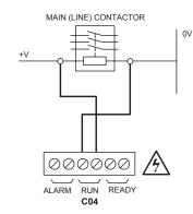
The RUN input will accept 12V to 250V ac (50/60Hz) only (DC cannot be used).
