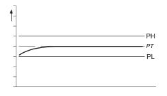
Where abrupt, or significant, changes in air demand, beyond the capacity scope of the variable capacity compressor, are experienced, the loading and unloading of other compressors is implemented in exactly the same way as described above. If demand for air is abruptly, or significantly, increased, and the capacity output of the compressor loaded at the Low Pressure set point (b) is insufficient, the pressure will continue to decrease at a reduced rate.
