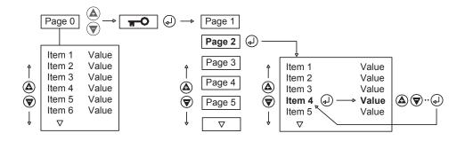
Press ESCAPE at any time in menu mode to step backwards one stage in the navigation process. Pressing ESCAPE when the page number is flashing will exit menu mode and return the display to normal operational mode.
