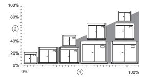
1: Demand 2: Generation Not all potential combinations are shown. Energy Control mode incorporates adaptive strategies and dynamic responses that continuously modify basic principles. With 'built-in' knowledge of individual compressor capabilities the management unit adapts to accommodate system characteristics under varying demand situations.
