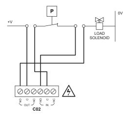
Three Wire Pressure Switch Connections:
