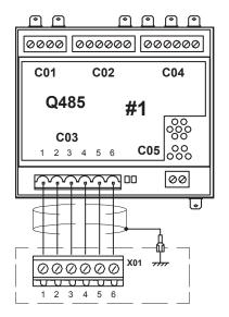
The 'Q485' is a DIN rail mountable module designed to be installed within the compressor control or switchgear area.
