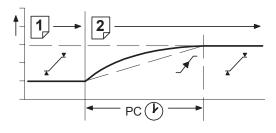
The time the system will take to complete the transition from one pressure target to another is determined by the 'Pressure Change' time (PC). This value can be adjusted to accommodate installation characteristics to achieve the transition at optimal energy efficiency.
