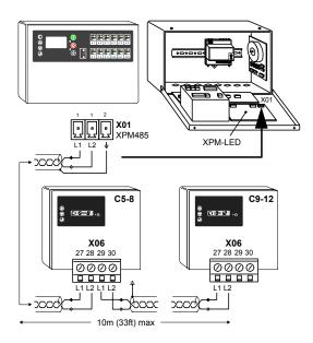
Use a twisted pair, earth shielded, 0.25mm2-1.0mm2 data communications cable with a total length no greater than 10m (33ft).
