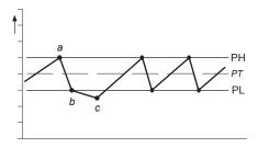
The same method is implemented in reverse (above the High Pressure set point) when an abrupt, or significant, decrease for air demand is experienced.
