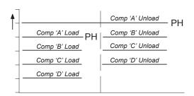
① The pressure set points are not dynamic and remain fixed and unchanging. The 'average' system pressure will decrease dependant on the number of compressor(s) running as demand increases.
