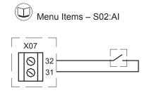
The input is designed to detect a remote 'voltfree' switching contact (rated for a minimum 24VDC @ 10mA).
