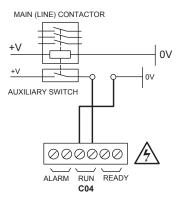
In instances where a motor starter contactor is not available or accessible, any part of a compressor control circuit that is energised when the compressor is running can be monitored. For example: fan contactor or voltage signal to a remote starter. (1) The 'Q485' input common terminal must always be connected to the neutral, common or 0V line of the applied input voltage.
