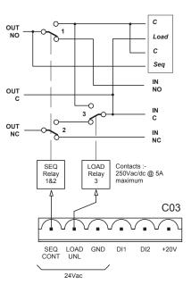
The C01 and C02 terminal functions of the 'Q485' are intended to control load and unload regulation of the compressor.
