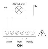
The Alarm input will accept 12V to 250V ac (50/60Hz) or dc.
