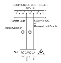
① Compressors that use electronic pressure detection but are not equipped with a remote pressure control enable feature will not automatically revert to local control if the Conductor 12 is stopped or experiences a fault or loss of power.
