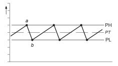
When system pressure increases to the High Pressure set point (a) a compressor is unloaded. Pressure is allowed to decrease to the Low Pressure set point (b) before a compressor is loaded again to add capacity output and increase pressure. This process will continue under a steady demand for air in a continuous stable cycle.
