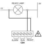
The READY input will accept 12V to 250V ac (50/60Hz) or dc.
