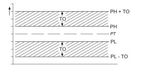
Tolerance (TO) is expressed as a pressure defining the width of the tolerance 'band'.
