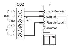
Examine the 'Q485' internal output circuit diagram to establish any desired switching logic that may differ from normal practise.
