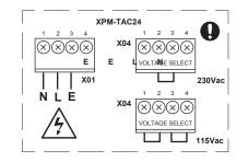
(1) Before applying power to the 'Direct Connect Gateway' Module ensure that the power supply connections are correct and secure and that the operating voltage selector is set correctly for the power supply voltage in use; 115Vac or 230Vac (+-10%), 50/60Hz.
