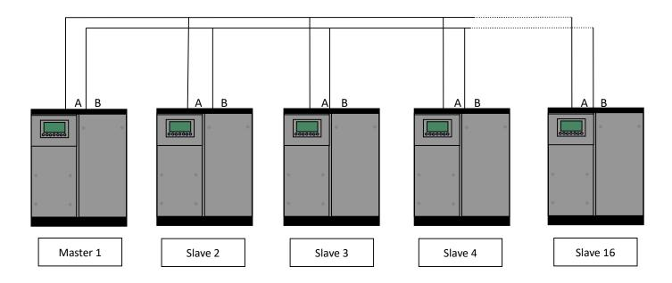
Compressors with net communication address 0001 is master, others are slave. Any one MAM-series compressors can be set as master or slave
